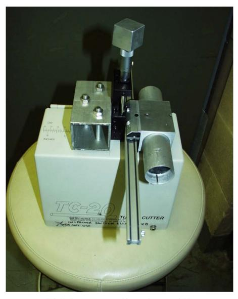
FIG. 27. Remote target cutter. Photograph courtesy of ANL.
