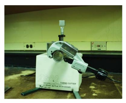
FIG. 29. Manual pipe cutter for making cuts at the ends of the target. Photograph courtesy of ANL.
