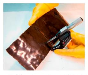
FIG. 8. Uranium metal foil fabricated on a trial basis by Y-12. The thickness of the foil is  $\sim$ 115  $\mu$ m.
