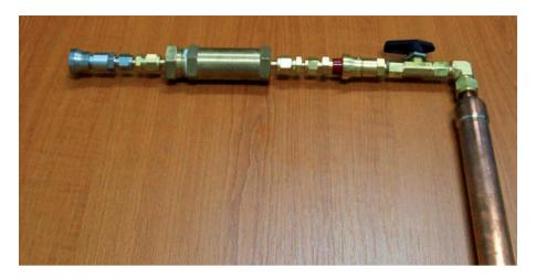
FIG. 52. Iodine and noble gases recovery device built by Romania.
