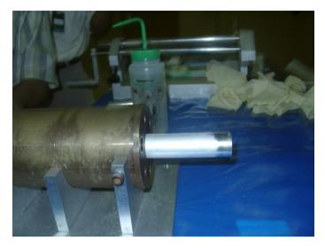
FIG. 17. Draw die assembly with target. Photograph courtesy of BATAN.
