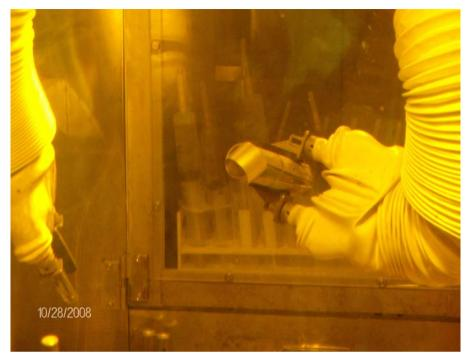
FIG. 15. LEU foil removal from aluminium tubes. Foil is being placed in dissolver unit.
