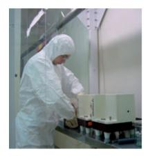
FIG. 73. Assembling of  $^{99m}$ Tc gel generators with  $Zr^{99}$ Mo gel in the clean module. Photograph courtesy of INP, Kazakhstan.
