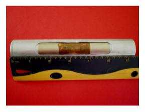
FIG. 5. Mock annular target shown with nickel wrapped 20 g copper foil exposed.
