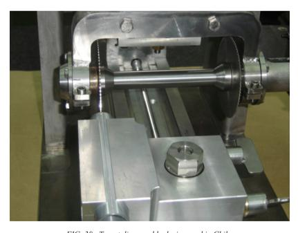
FIG. 38. Target disassembly device used in Chile.
