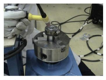
FIG. 20. Performing the welding of the two tubes. Photograph courtesy of BATAN.
