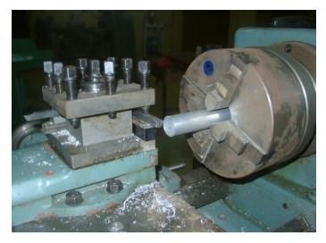
FIG. 19. Machining the ends of the tubes in preparation for the weld. Photograph courtesy of BATAN.
