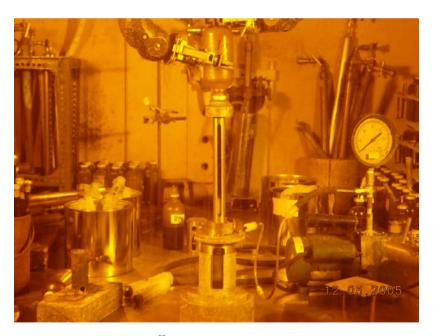
FIG. 55. Purification of <sup>99</sup>Mo by HZO column at PUSPIPTEK, Indonesia.
