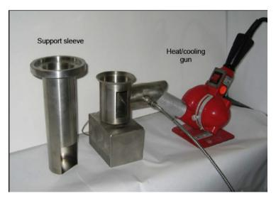
FIG. 44. Dissolver for LEU modified Cintichem heater and support. Photograph courtesy of ANL.
