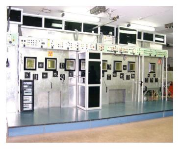
FIG. 64. Gel generator production facility at BRIT, India — the hot cell windows are visible. Photograph courtesy of BRIT, India.
