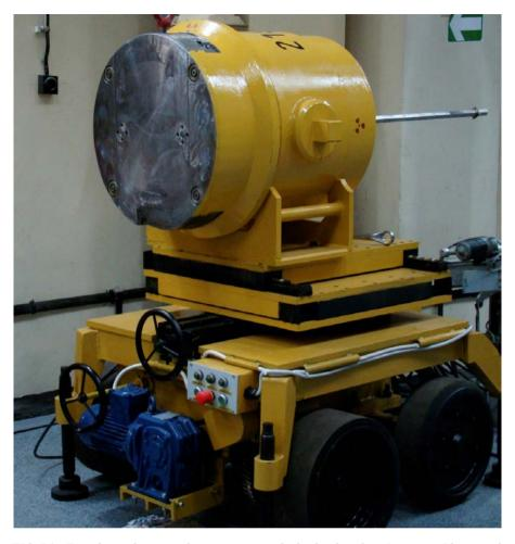
FIG. 76. Transfer cask mounted on transport vehicle developed in Romania. Photograph courtesy of ICN.
