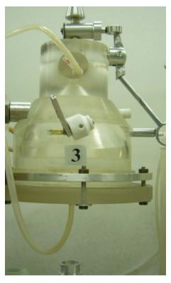
FIG. 71. Equipment for filtration, drying and filling of dried gel granules. Photograph courtesy of INP, Kazakhstan.
