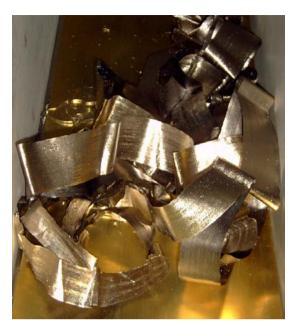
FIG. 10. Foils as they were ejected from the cooling roll. Photograph courtesy of KAERI.
