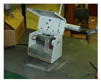
FIG. 28. Remote target cutter. Photograph courtesy of ANL.
