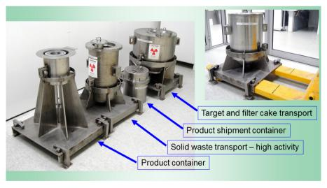
FIG. 75. Transport casks for different duties within the <sup>99</sup>Mo production process at PINSTECH. Courtesy of GSG.
