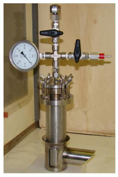
FIG. 47. New foil dissolver, Romania.
