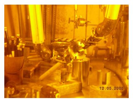
FIG. 56. Foil being placed in the dissolver at PUSPIPTEK, Indonesia.
