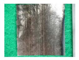
FIG. 12. Uranium metal foil fabricated by KAERI using their cooling roll casting method. The average thickness of the foil is ~140 µm. Photograph courtesy of KAERI.
