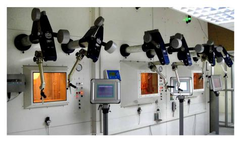
FIG. 62. <sup>99</sup>Mo production hot cell facility at PINSTECH in Pakistan. Photograph courtesy of GSG.
