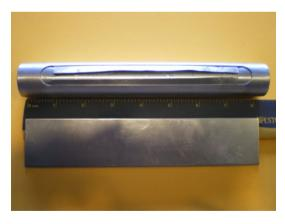
FIG. 6. LEU foil annular target comparison to an HEU based  $UAl_x$  dispersion target used by Covidien/Mallinckrodt.
