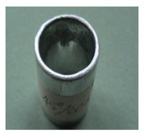
FIG. 21. Final welded target. Photograph courtesy of BATAN.
