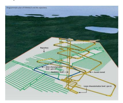
*Figure 1*: Diagrammatic plan of ONKALO and the repository. Reprinted from Programme of monitoring at Olkiluoto during construction and operation of the ONKALO. Posiva Oy Report (2003), p. 5.
