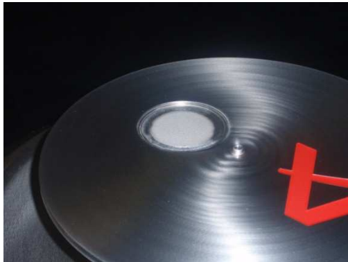
Figure 3.4 Poral filter in the cover of a canister
