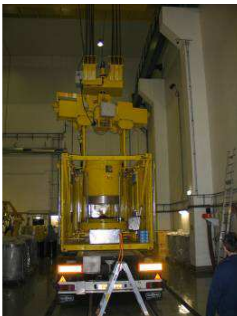
Figure 1.5 The unloading of an MTR-2 container with research reactor fuel elements (RR-HPW)
