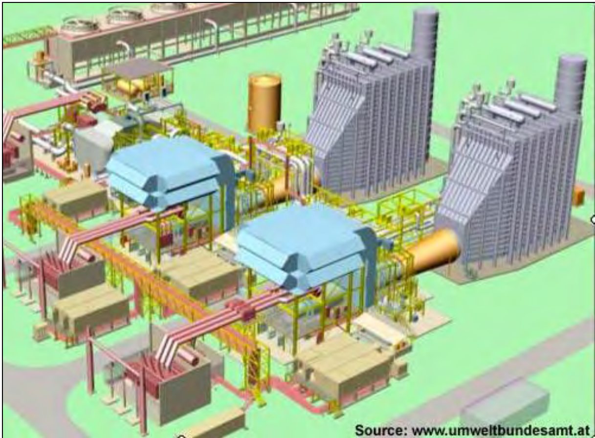
Figure C-4: Combined Cycle Power Plant General Arrangement
