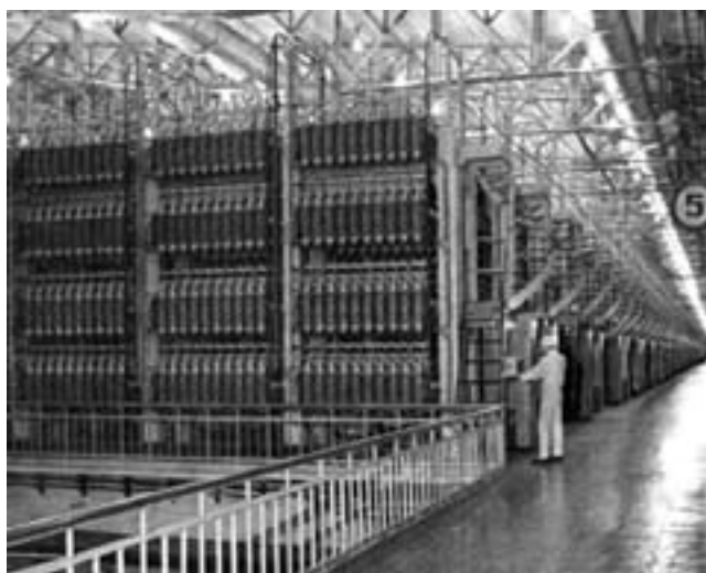
Figure 8.2. Centrifuge cascade in the Novouralsk centrifuge enrichment plant. Russian centrifuges are short and stacked on top of each other. 386
