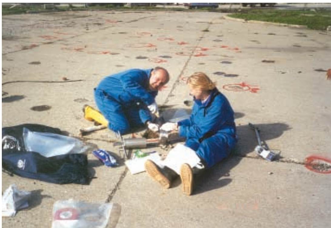
Sampling penetrator impacts in the concrete platform at the Djakovica/Djakovica garrison. The penetrator hits are marked by red spray paint.
