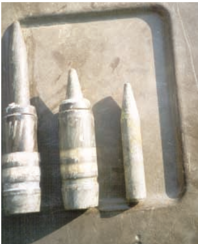
One penetrator (right) and two penetrators still fixed in their jackets. The left penetrator has partly moved from its position in the jacket. The length of the penetrator is 95 mm.
